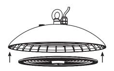
6. Fasten the new lens with the screws that were removed at STEP 1.
