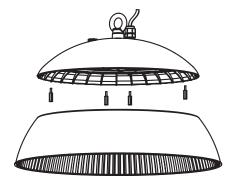
3. Fasten the 4 screws on to the studs.
