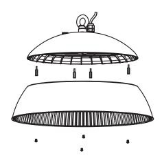
4. The install of the PC reflector is completed.
